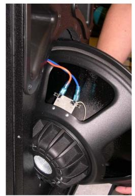
Figure 1. The orange wire connects to the + terminal, and the blue wire to the - terminal.
